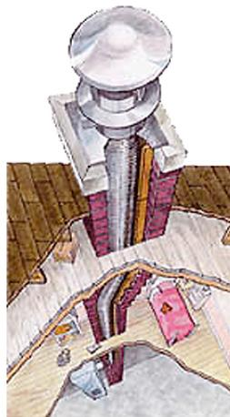
some cases, the chimney liner may have to be replaced to reduce the risk of backdrafting. If you have a gas furnace with a masonry chimney, you must have a metallic liner. Have your contractor inspect for this.
