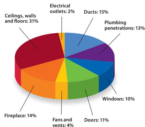
Air infiltrates into your home through every hole, nook and cranny. About one-third of this air infiltrates through the openings in your ceilings, walls and floors.
