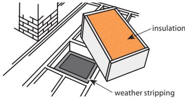
If you have an attic hatch, make sure it fits tightly and is backed by insulation. Do this by weather-stripping the edges of the access hole and building a simple wood box to hold insulation on the backside of the hatch.
