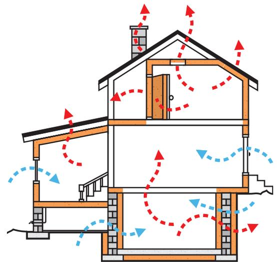
Plugging air leaks after a careful inspection of your home's structure—both inside and outside—can yield a significant reduction on your monthly heating and cooling bill. In this illustration, blue arrows indicate outside air infiltration and red arrows show where conditioned (heated or cooled) air can escape.
