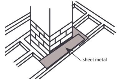
Heat can escape around the chimney, if it isn't properly sealed.
