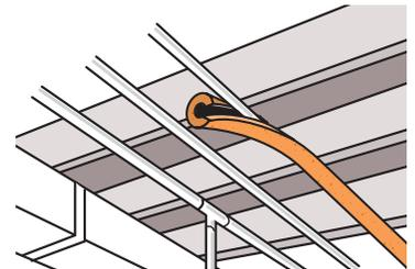
Use foam insulation on hot water pipes in your basement or crawl space. The water will stay warmer in the pipes, cutting the time you need to wait for hot water for sinks, bathtubs or showers.
