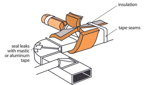
Tighten and seal leaky ducts before insulating with foil- or paper-faced batts made especially for ducts.
