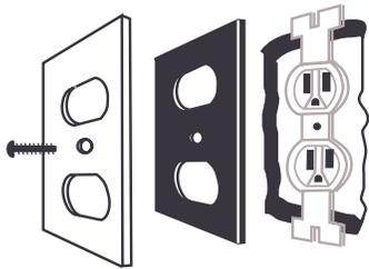
Install outlet gaskets between the electrical outlet and the coverplate. Plastic plugs—such as “child safety” inserts—also will prevent air from entering your home.
