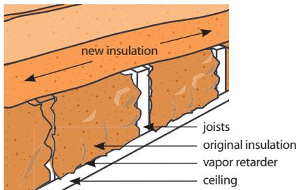
When you add insulation to your attic, run the new batts perpendicular to the direction of the ceiling joists to cover air gaps that may have developed in the existing insulation along the joists.
