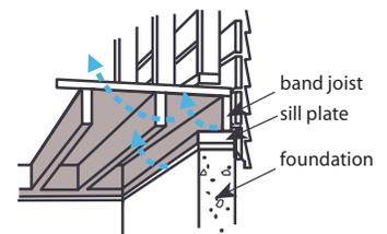
Get rid of drafts on the main floor by caulking along the sill plate and band joist in the basement.
