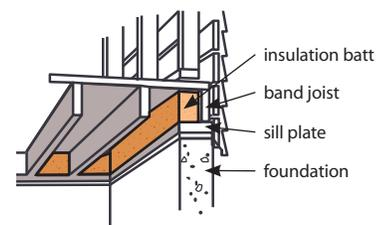
Cut insulation to fit band joist spaces between the sill and subfloor.
