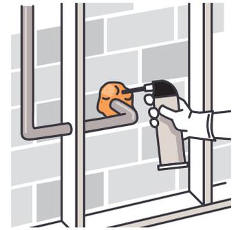
Expanding foam sealant works well for sealing gaps more than 1/4 wide.
