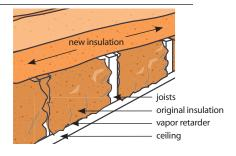
When you add insulation to your attic, run the new batts perpendicular to the direction of the ceiling joists to cover air gaps that may have developed in the existing insulation along the joists.
