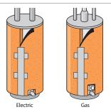
Giving your water heater a blanket to lower your water-heating bills is an easy, do-it-yourself job. Be sure to follow the insulation manufacturer's installation instructions—the process differs for electric and gas water heaters.
