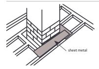
Heat can escape around the chimney, if it isn't properly sealed.
