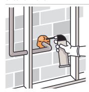
Expanding foam sealant works well for sealing gaps more than 1/4 wide.
