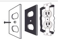
Install outlet gaskets between the electrical outlet and the coverplate. Plastic plugs—such as "child safety" inserts—also will prevent air from entering your home.
