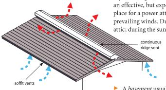
If you're reroofing or building a new home, a continuous ridge vent combined with soffit vents offers optimal attic ventilation. In this illustration, blue arrows indicate outside air flowing into the attic and red arrows show attic air flowing out.
